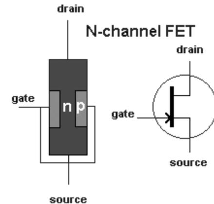
In a field effect transistor, the **gate** controls the conductance of the channel, the **source** is where the charge carriers enter the channel and the **drain** is where the charge carriers leave the channel.
