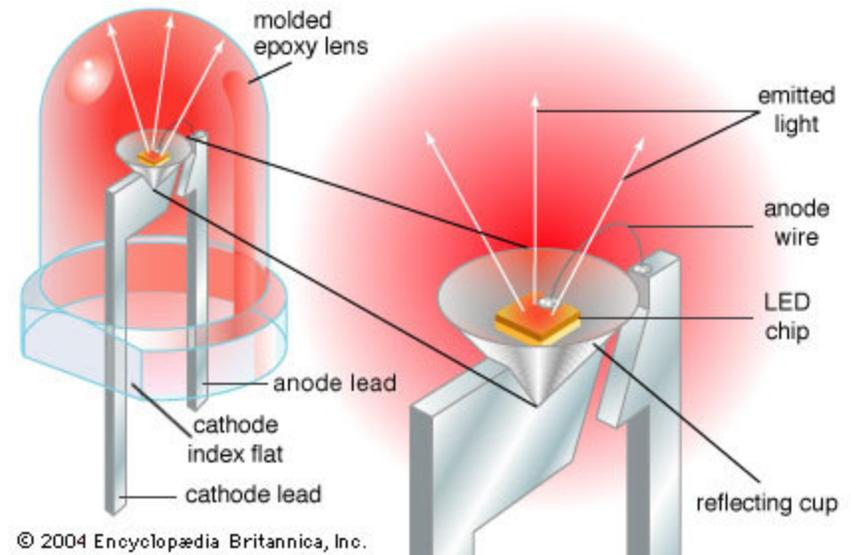
LEDs are made of various semiconducting compounds, depending on the desired colour output. Infrared and red LEDs generally use a gallium, aluminum, and arsenide compound. Orange and yellow LEDs most often use gallium, aluminum, and either indium or phosphorus. Green and blue LEDs typically use either silicon and carbon, or gallium and nitrogen.
